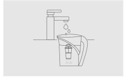
Fill top section with water and allow to flow through filter. Discard water and repeat once. The filter is now activated and ready for use.
