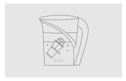
Submerge filter under cold tap water, gently shake to remove air bubbles and leave to soak for 5 minutes. Note: remove the funnel section of the jug and submerge the filter inside the jug or alternatively use the sink.
