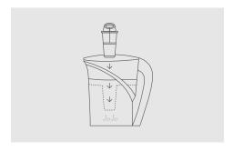
Insert funnel into the jug (if removed for Step 1). Place filter into the hollow of the funnel and push downwards until positioned firmly.
