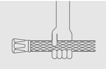
Disconnect existing 1/2" copper pipe/stainless steel braided hose at the stop cock, and insert 3/4 multifunctional valve **(6)**.
