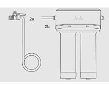
Fit one end to the filter isolating valve (7). Insert the other end into the quick connector of the filter inlet (4) by first removing the blue retaining clip (12), then inserting the tube and replacing the clip.
