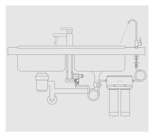
Let the system run for a few minutes to flush the cartridges. Allow the system to stand for 2 to 3 hours and flush again for several minutes. Your filter is now ready to be used and you can enjoy clean, safe and great-tasting water.
