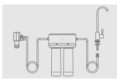
Once all the tubing has been connected (from multifunctional valve to inlet, and from outlet to chrome-plated tap), place the chrome-plated tap in the open position, then open filter isolating valve (7) slowly. This will allow any air to escape. Check for any leaks and adjust if necessary.
