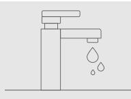
Isolate water supply to your kitchen tap. Turn on kitchen tap to release pressure in pipe then turn tap off.
