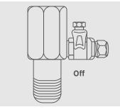
The valve should be in the off position. Turn the water supply on, then slowly turn the kitchen tap on and check for leaks.
