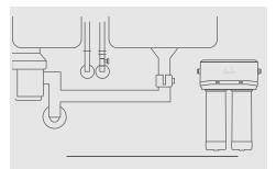
Find a convenient location for the filter under the sink. *Note:* consider ease of access for servicing and best use of cupboard space.
