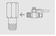
Install filter isolation valve (7) into the multifunctional valve.
