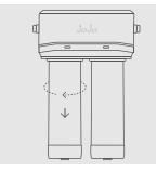
To remove filters, turn each filter 1/4 turn to the left and pull downwards. *Note:* on the filters there are indicators of which way to turn it in order to lock or release the unit.
