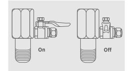
Turn filter isolating valve off and open filter's chrome-plated tap to release pressure.
