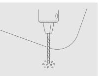
Drill 3mm pilot hole, then drill 12mm final hole. *Note:* use a slow speed drill as excessive speed may blunt the drill and/or discolour stainless steel.
