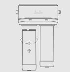
To replace the filters, insert each filter into the correct slot and turn 1/4 to the right until it stops to ensure it is firmly in place.
