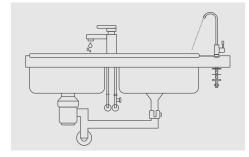
Slowly turn on the filter's isolating valve to expel air and initial water flush. Let the system run for a few minutes to flush the cartridges. Allow the system to stand for 2 to 3 hours and flush again for several minutes.
