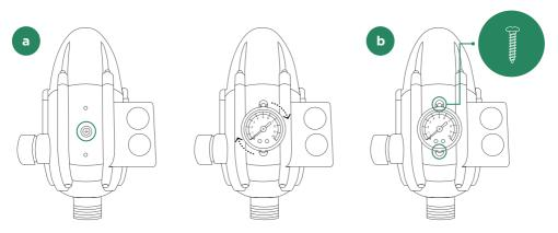
b. Firmly secure the pressure gauge (2) in place by using the screws (3) provided. Ensure that it is flush against the flow controller (1) to prevent leakage.
