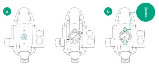
**b.** Firmly secure the pressure gauge **(2)** in place by using the screws **(3)** provided. Ensure that it is flush against the flow controller **(1)** to prevent leakage.
